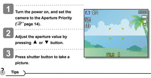
The larger the aperture value the smaller the lens opening, allowing less light to enter the camera.
