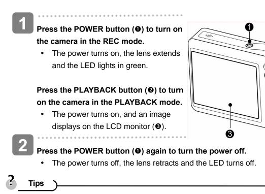
You can turn on the camera without the start-up and operating sound by pressing and holding the POWER (●) or the PLAYBACK (●) button over 1.5 seconds.
