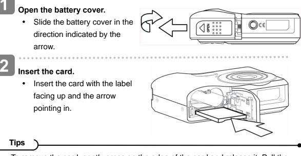
• To remove the card, gently press on the edge of the card and release it. Pull the card out and close the battery cover.
